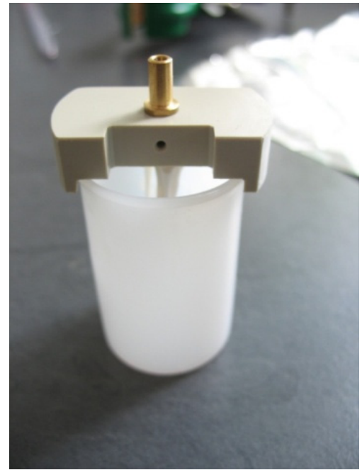
Fig. (1). Photo of the experimental set-up: The implant was fixed in a custom made device, permitting coaxial alignment and then embedded in a polyester resin.
